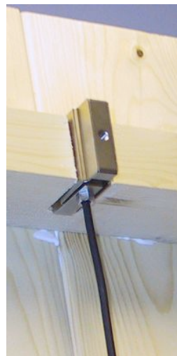
Floor with embedded S-load cell
